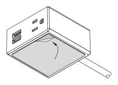
Remove plastic film from the microsuction pad and place on a clean, smooth surface.
